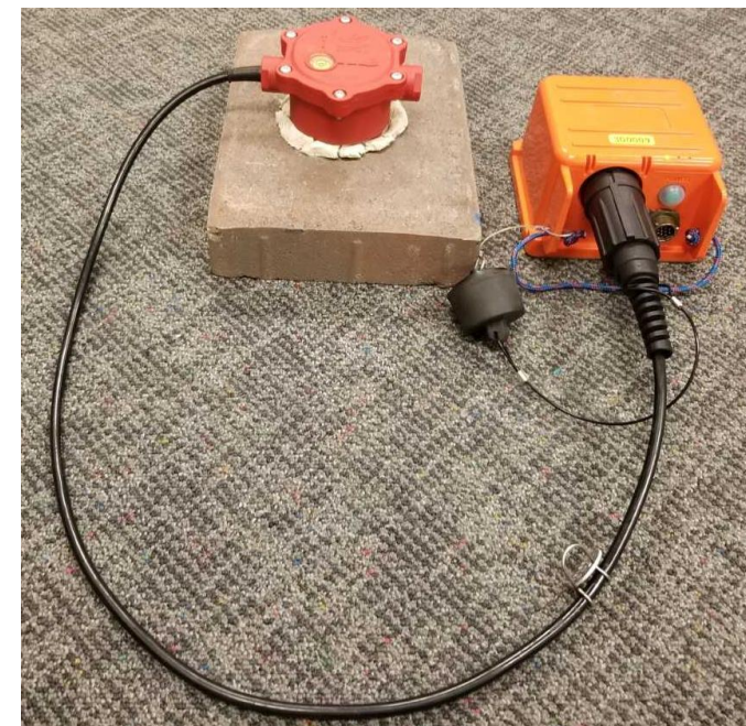
3C Atom and 3C 2Hz geophone at Geometrics office, San Jose, CA, U.S.
